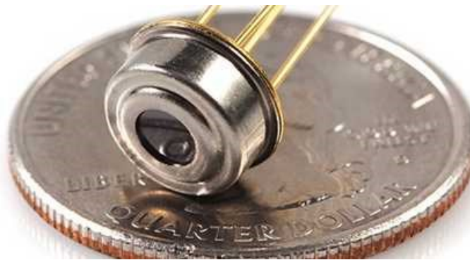
A long-wave IR temperature sensor. The longer wavelength requires a larger sensing region than visible or near-IR applications.
