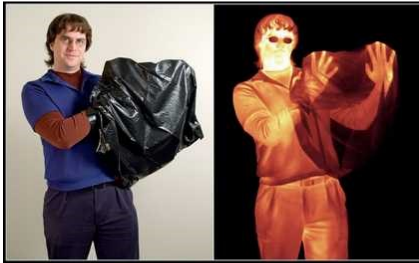
The same scene in the visible spectrum and the long-wavelength infrared. Notice that the plastic bag is opaque to visible light but nearly transparent to infrared (courtesy NASA Spitzer Infrared Telescope team).
